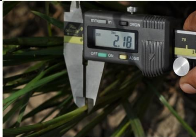
Figure 4. Culm diameter measurement using vernier caliper
