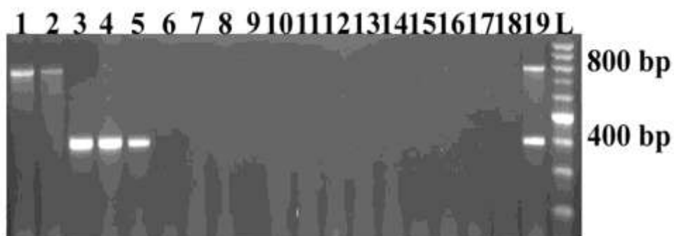
Figure 1. Identification of cytoplasm types in maize inbred lines by PCR. Lanes 1 to 18 correspond to inbred lines mentioned in Table 1. Lane 19: positive control includes DNA from inbred lines 1, 3 and 8. L: 100 bp ladder.
